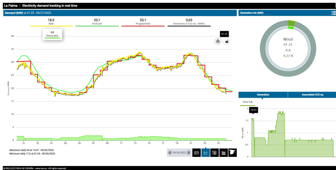
Figure 2-11 Demand forecast, scheduled demand, real demand and aggregated ND-RES generation of the island power system of La Palma - September 26, 2022. Source: [12]
